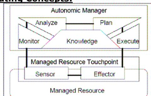
Figure 1. Autonomic Computing Control Loop
